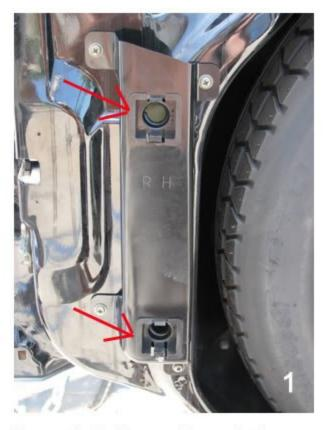
Remove the inside spare tire panel, Then pop the plastic square inserts out of the panel hanger.
