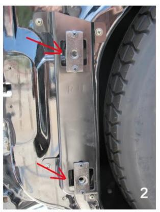
You will line up the new bolt hangers directly in the middle of the square holes and attach by using the supplied self tapping screws. Refer to pic #3
