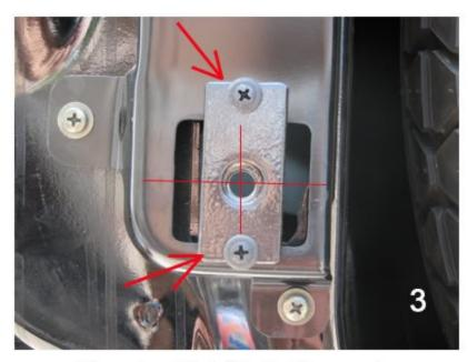
The center of the bolt is offset to one end.
